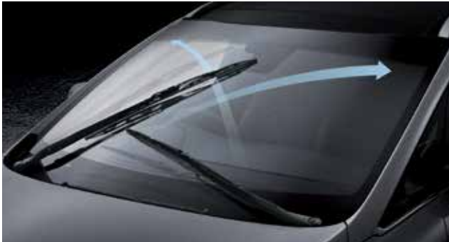
Opposed-type wiper system Unlike conventional wiper systems, the wiper blades are mounted on opposite sides of the windshield and move in the opposite direction for maximum visibility even in heavy rain and snow.
