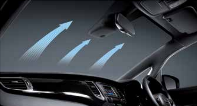
Auto defogging system A sensor automatically initiates a defogging process when condensation is detected on the windows to ensuring optimal visibility in humid climates.
