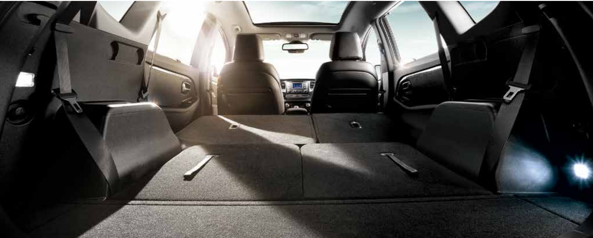
Spacious cargo room A walk-in sliding function on the second-row seats enables occupants to access the third row with a light touch of a lever, while the flat-folding configuration provides expansive space for all types of cargo.
