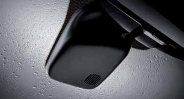
Rain sensor The windscreen wipers are automatically activated as soon as moisture is detected for greater convenience and visibility.
